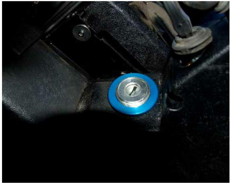
Screw the Blue Aluminium Bezel over the thread on the column sleeve. A little grease on the threads makes this much easier as the threads are deliberately tight. If you find you cannot grip the bezel tightly enough, wrap some tape, sticky side out round your finger tips. This will help you grip the bezel without damaging it.
